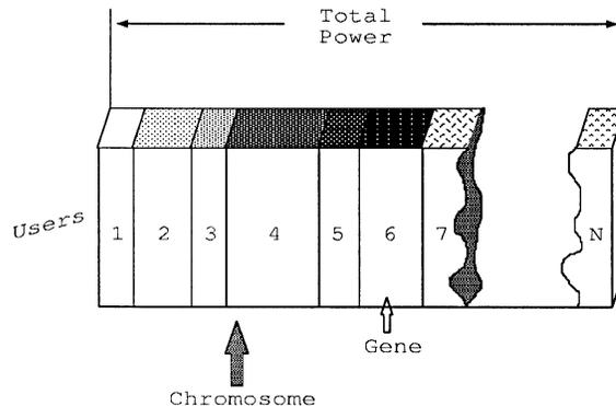
Fig. 3 Power allocation issue in a DS-CDMA cellular system.
