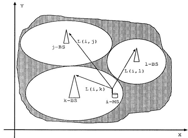
Fig. 1 A typical case [1] of wireless cellular geometry.
