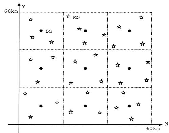
Fig. 2 A large-scale DS-CDMA cellular system.
