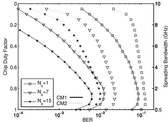
**Fig. 3** BER performance vs. DF for DS-UWB system.  $T_c$  is set to constant 4 ns with  $0.04 \text{ ns} \leq T_p \leq 4 \text{ ns}$ . SNR=20 dB,  $L_c=8$ ,  $f_c=4 \text{ GHz}$ .
