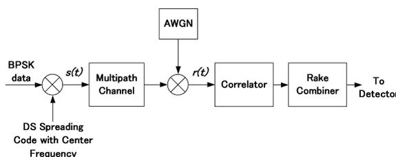
Fig. 1 System diagram of DS-UWB system.
