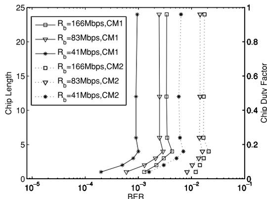
**Fig. 2** BER performance vs. DF and chip length for DS-UWB system. SNR=20 dB,  $L_c=8$ ,  $f_c=4$  GHz.
