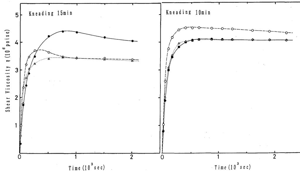
Fig. 3. True viscosity developments of rice cake samples of various varieties. The shear rate was  $1.78 \times 10^{-3}$ , the kneading times were 10 min and 15 min and the measurement was carried out at  $90^\circ\text{C}$ . ●, K; △, H; ○, T.
