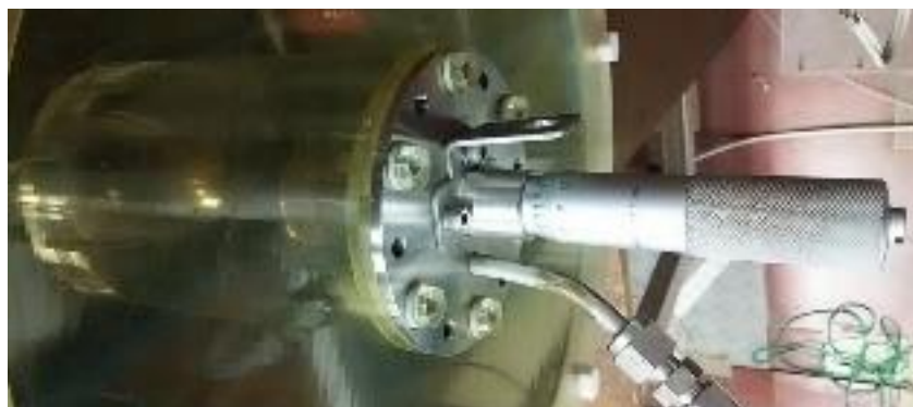
Fig. 2.18 Gap-switch with the adjusting handle.
