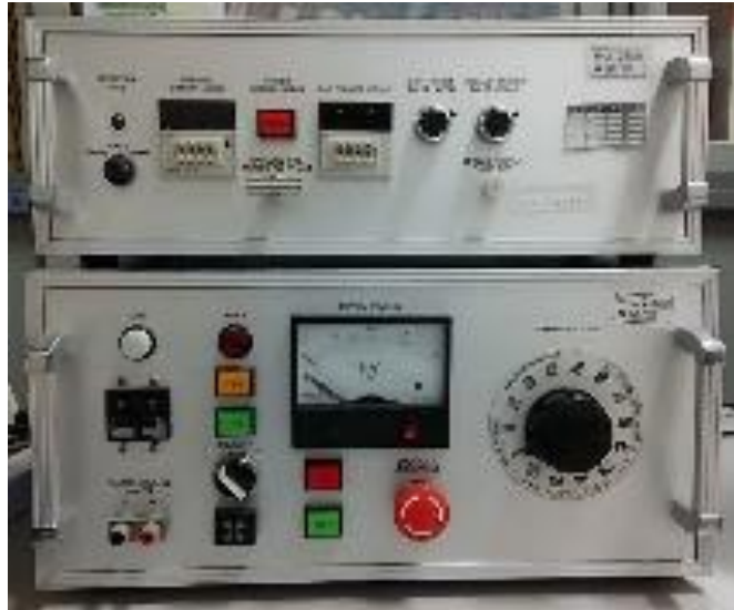
Fig. 2.17 Sequence controller for the Marx generator charging control.
