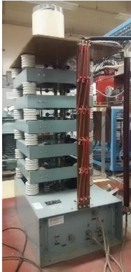
Fig. 2.3 Photograph of the Marx generator.
