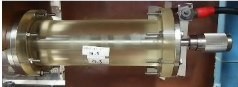
Fig. 2.19 Electron beam current control handle.
