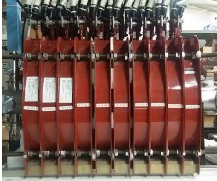
Fig. 2.10 Photograph of magnetic field coils.
