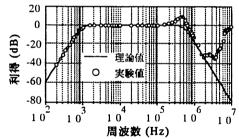
図 6 振幅特性 1  $(\omega_L = 2\pi \times 1 \times 10^{-1} \text{ rad/s}, \omega_H = 2\pi \times 500 \times 10^{-1} \text{ rad/s})$
