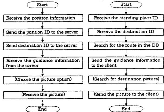
Figure 2 User terminal part Figure 3 DB server part
