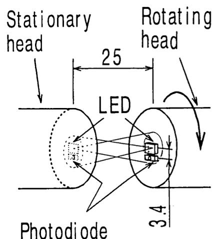
Fig.2 Arrangement of the optical devices.
