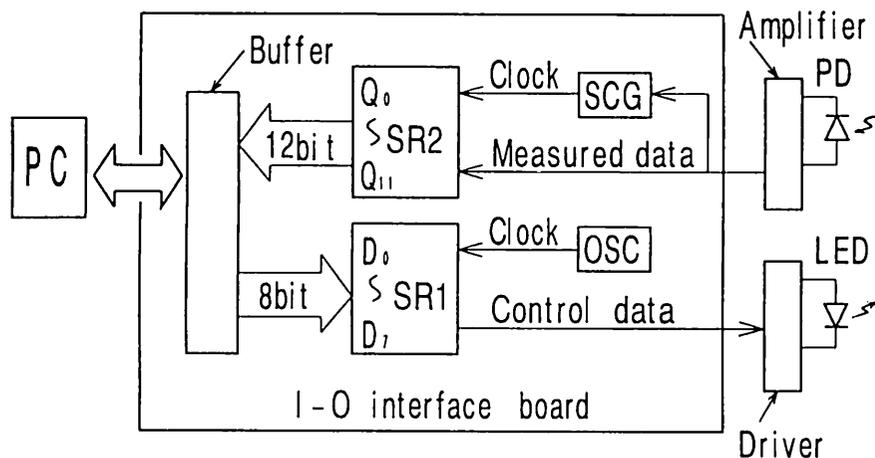
Fig.3 Block diagram of the I-O interface board.
