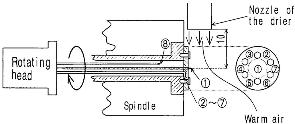
Fig.8 Experimental setup and the measurement positions of temperature.
