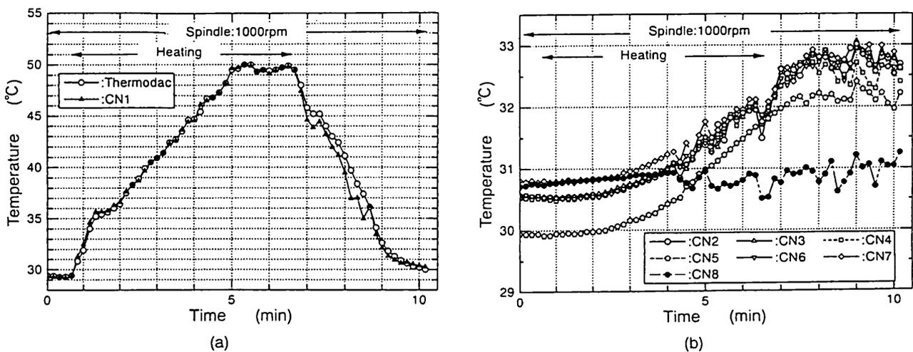
Fig.9 Temperatures measured with (a) CN1 and Thermodac, and (b) CN2 ~ CN8.
