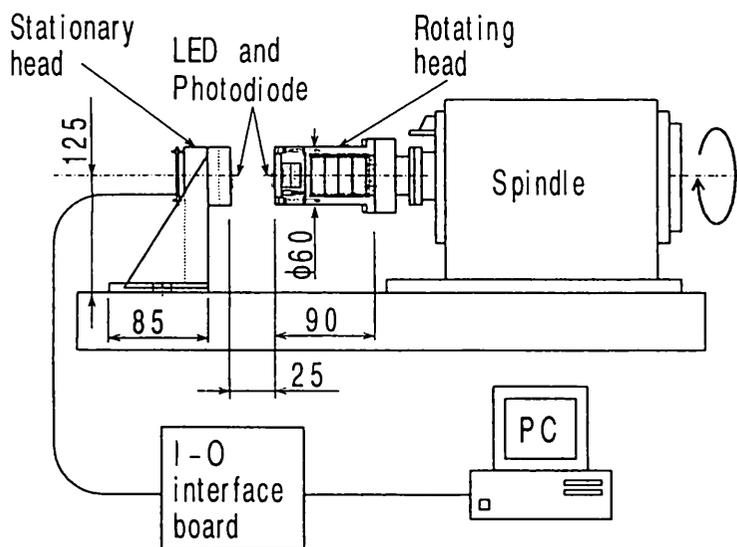
Fig.1 Optical telemetering system.
