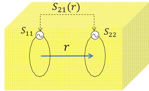
Fig. 1. The Position and Distance for Two Insulated Circular Loop Antennas (ICLAs) Faced in the Tissue-Equivalent Liquid to Calibrate the Near-Field Gain
