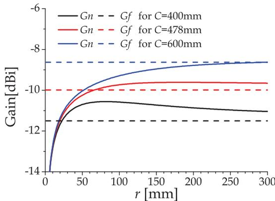
Fig. 3. Distance Dependence of Simulated Near- and Far-Field Gain of the Insulated Circular Loop Antenna (ICLA) with the circumference of  $C = 400$  mm, 478 mm, and 600 mm in the Tissue-Equivalent Liquid at 30 MHz
