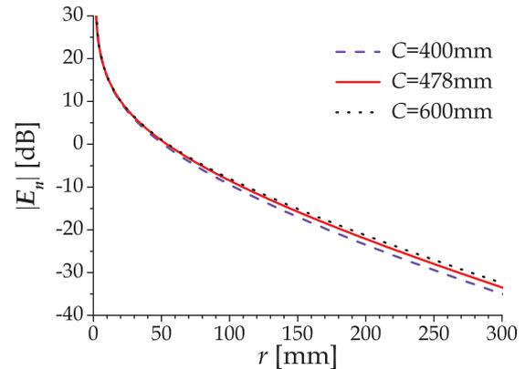
Fig. 5. Distance Dependence of Simulated Electric Field Intensity,  $|E_n(r)|$ , defined as (5), of the Insulated Circular Loop Antenna (ICLA) with the circumference of  $C = 400$  mm, 478 mm, and 600 mm in the Tissue-Equivalent Liquid at 30 MHz
