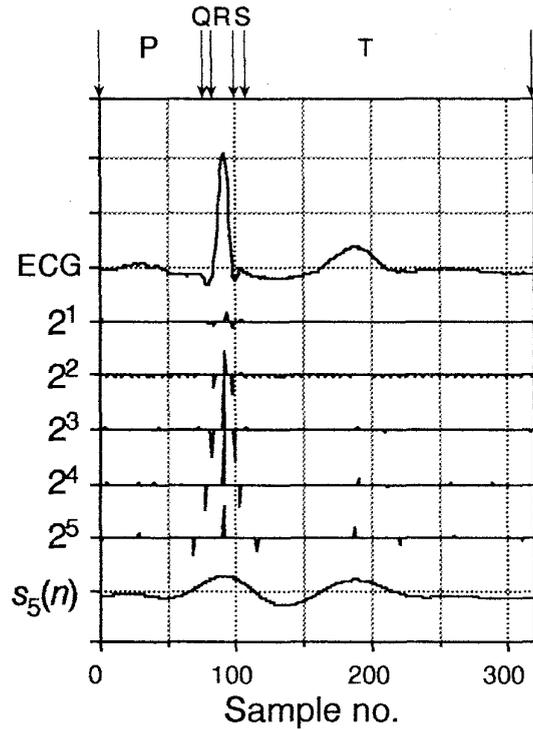
Fig. 1 Multiscale peak analysis of an ECG waveform
