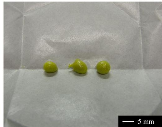
Fig. 4. Photographic image of the melted YAG phosphor samples.
