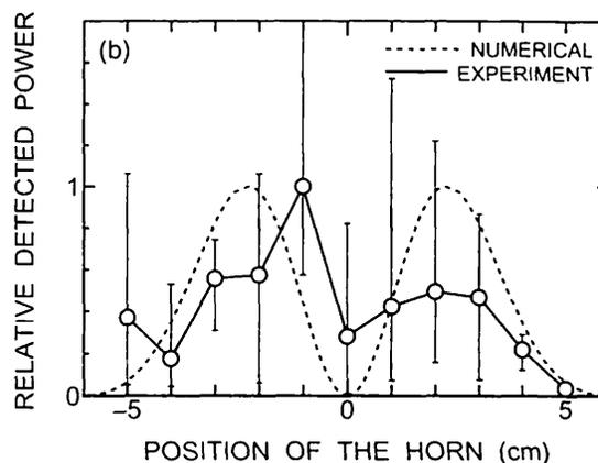
FIG. 3. (a) A typical shot of microwave signals. The delayed signal is obtained by using a 20-m-long waveguide delay line. (b) Radiation pattern of the output microwave obtained by scanning the receiving antenna vertically from the axis of the slow wave ECM.
