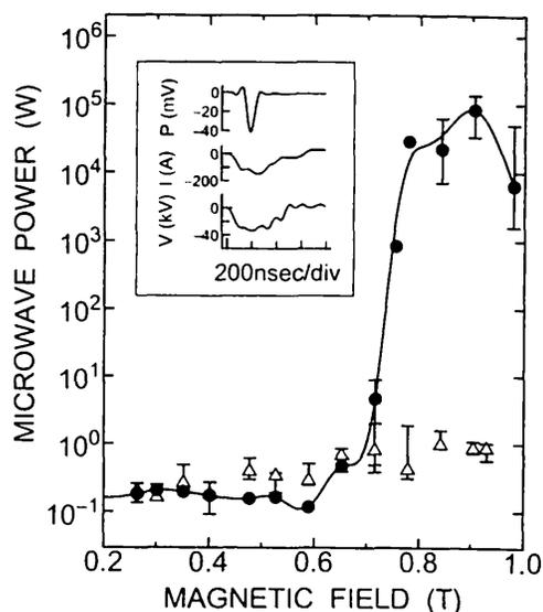
FIG. 2. Microwave output power vs applied axial magnetic field. Closed circles connected by solid line show absolute output powers of the slow-wave ECM. Open triangles are output powers when the periodic SWS is replaced by the straight cylinder waveguide with the same radius as the mean radius of the SWS. Inset shows the timing and wave forms of detected voltage of microwave power  $P$ , beam current  $I$ , and beam voltage  $V$ .
