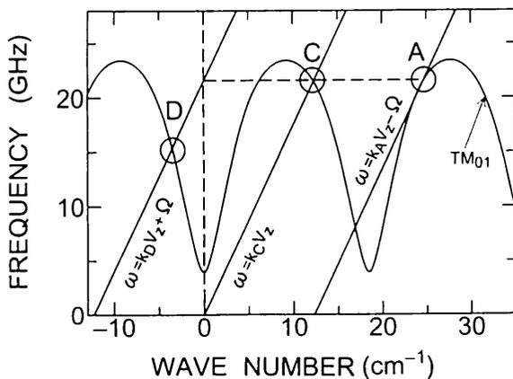
FIG. 4. The dispersion characteristics of the slow-wave ECM at the axial magnetic field of 0.76 T for the beam energy of 35 keV.
