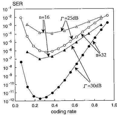
**Fig. 1** SER vs. coding rate of the PC/SS system in Rayleigh fading channel ( $M=16$ ,  $r=2$ ,  $k=8$ ).
