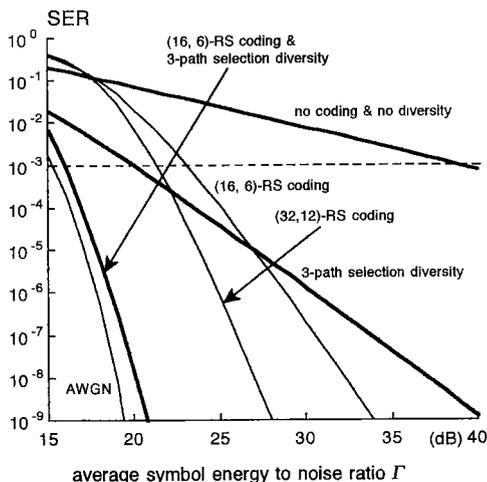
**Fig. 3** SER of PC/SS system with 3-path selection diversity ( $M=16$ ,  $r=2$ ,  $k=8$ ).
