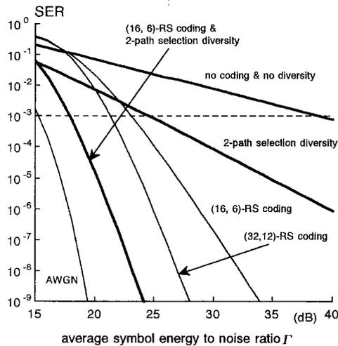
**Fig. 2** SER of PC/SS system with 2-path selection diversity ( $M=16$ ,  $r=2$ ,  $k=8$ ).
