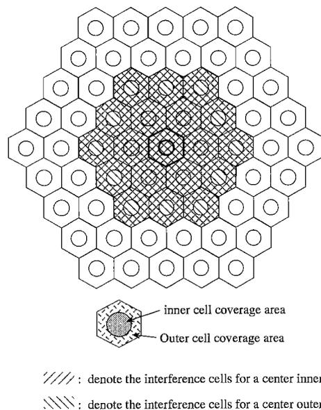
Fig. 1 Illustration of a Reuse Partitioning system and representation of the structures of the interference cells.
