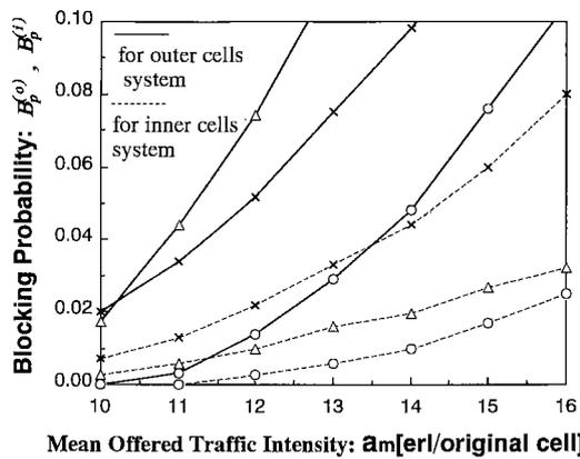
(b) blocking probability in the outer cells system:  $B_p^{(o)}$  and in the inner cells system:  $B_p^{(i)}$  for using the DCA rule with the channel division.
