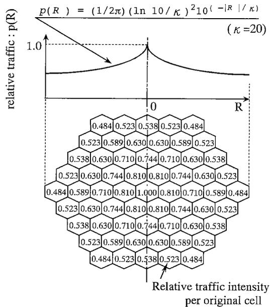
**Fig. 4** The model of inhomogeneous traffic distribution.
