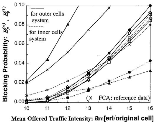
(c) blocking probability in the outer cells system:  $B_p^{(o)}$  and in the inner cells system:  $B_p^{(i)}$  for using the DCA rule without the channel division.
