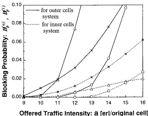
(b) blocking probability in the outer cells system:  $B_p^{(o)}$  and in the inner cells system:  $B_p^{(i)}$
