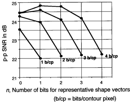
Fig. 5 Relation between the number of bits for a representative vector and the reconstruction precision.
