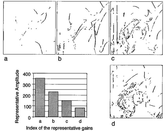
Fig. 3 Contour clustering by the gain of multiscale gradient vectors.
