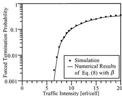
(d) Forced termination probability in the 2-belt buffering systems with 84 channels
