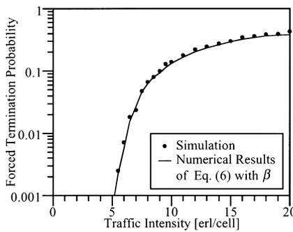
(b) Forced termination probability in the 1-belt buffering systems with 36 channels
