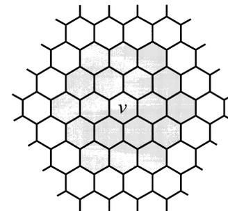
Interference cell of cell  $v$
