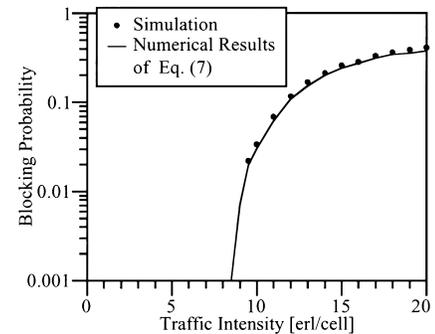
(c) Blocking probability in the 2-belt buffering systems with 84 channels
