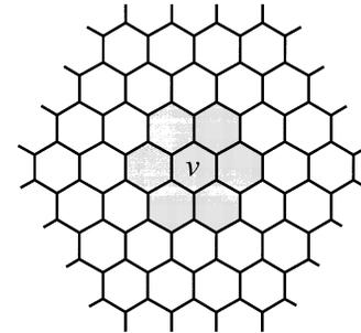
Interference cell of cell  $v$
