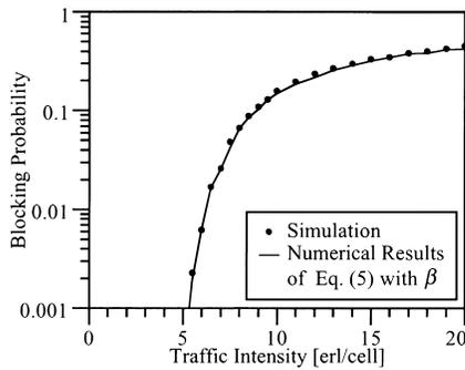
(a) Blocking probability in the 1-belt buffering systems with 36 channels
