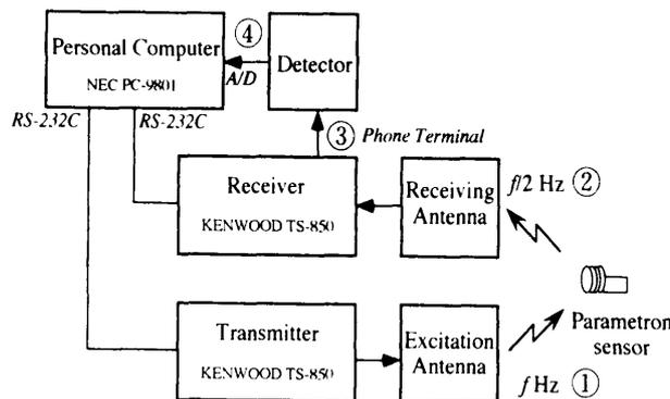
Fig. 3 Measurement system.
