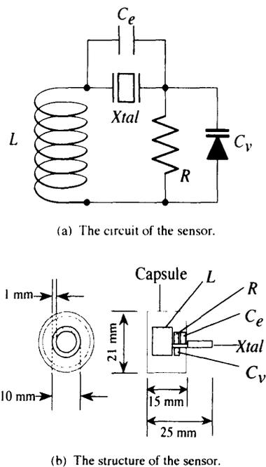
Fig. 1 Parametron-temperature sensor.  $C_e$ : Capacitor.  $C_v$ : Varactor.  $L$ : Coil.  $R$ : Resistor.  $Xtal$ : Quartz resonator.
