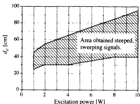
Fig. 9 Characteristics between excitation power and  $d_e$ .  $d_e$ : Distance between the sensor and the excitation antenna.
