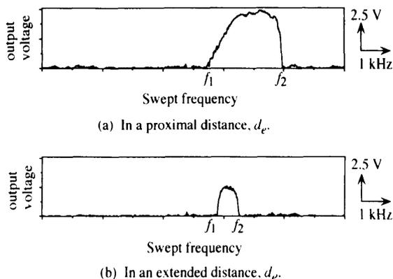
Fig. 8 Detected outputs of the receiver.  $d_e$ : Distance between the sensor and the excitation antenna.
