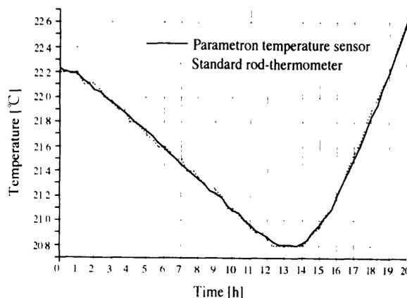
Fig. 11 Long-time measurement of temperature in a phantom.
