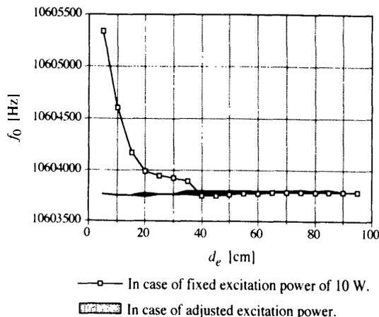
Fig. 10 Characteristics between  $d_e$  and  $f_0$ .  $d_e$ : Distance between the sensor and the excitation antenna.  $f_0$ : Oscillation-center frequency.
