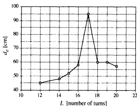
**Fig. 5** Characteristics of  $L$  vs.  $d_e$ .  $L$ : Coil.  $d_e$ : Distance between the sensor and the excitation antenna. Excitation power = 10 W.
