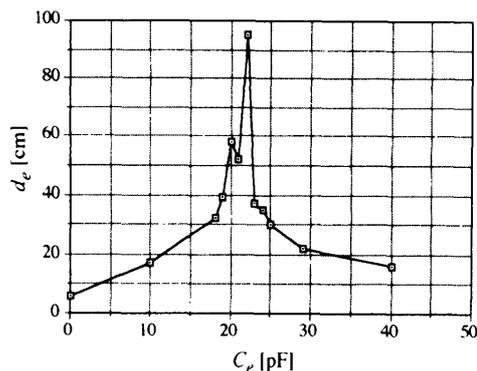
**Fig. 4** Characteristics of  $C_e$  vs.  $d_e$ .  $C_e$ : Capacitance of the capacitor.  $d_e$ : Distance between the sensor and the excitation antenna. Excitation power = 10 W.
