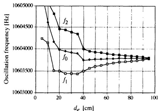
**Fig. 6** Characteristics between  $d_e$  and oscillation frequency.  $d_e$ : Distance between the sensor and the excitation antenna.  $f_1$ : Oscillation-start frequency.  $f_2$ : Oscillation-stop frequency.  $f_0$ : Oscillation-center frequency. Excitation power = 10 W.
