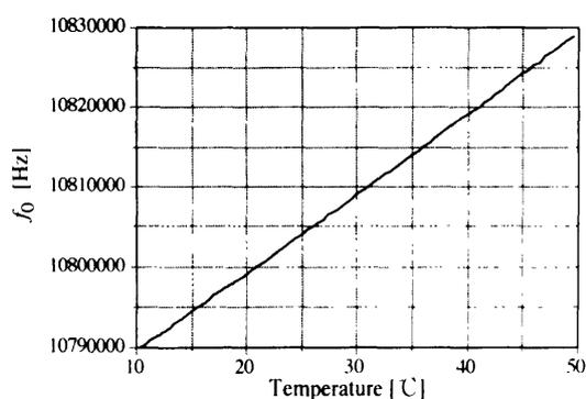
**Fig. 7** Relationship between temperature and  $f_0$ .  $f_0$ : Oscillation center frequency. Excitation power = 10 W.
