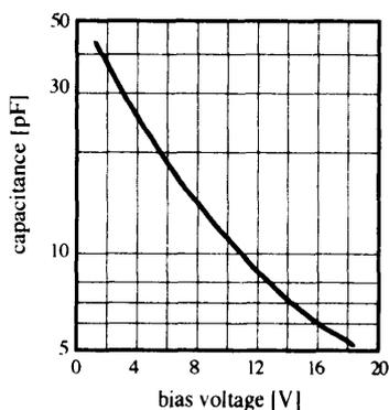
Fig. 2 Relationship between bias voltage and the capacitance of a varactor (SV101).
