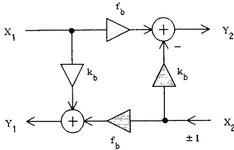
Fig. 7 Simplified realization of the constant lossless section.
