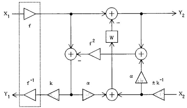
Fig. 5 Unified realization of basic transfer matrices.
