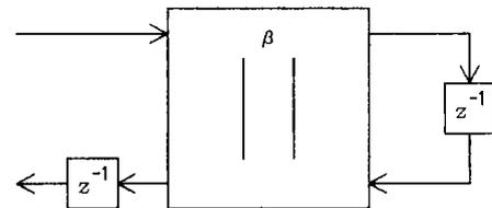
Fig. 6 Realization of the second-degree delay function block by a two-port adaptor.
