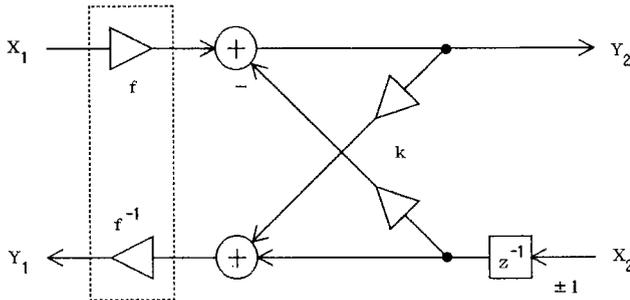
Fig. 8 Lattice realization of the first-degree section for the transmission zero at  $z=0$ .
