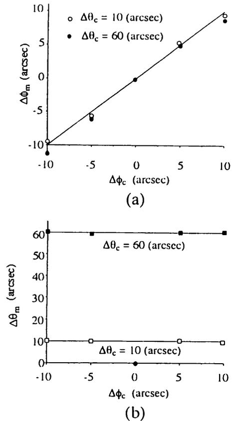
Fig. 7. Measurement results of errors  $E_{\Delta\phi}$  and  $E_{\Delta\theta}$  at  $\Delta\theta_c = 10$  and  $60$  arcsec, respectively.
