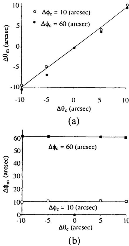
Fig. 8. Measurement results of errors  $E_{\Delta\theta}$  and  $E_{\Delta\phi}$  at  $\Delta\phi_c = 10$  and 60 arcsec, respectively.
