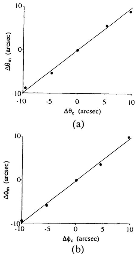
Fig. 9. Measurement results of 2D small rotation angles  $\Delta\phi$ ,  $\Delta\theta$  within  $\pm 10$  arcsec.
