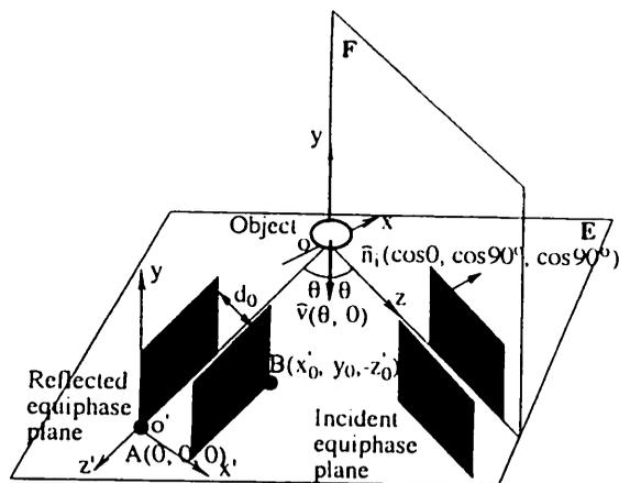
Fig. 4. Ideal configuration for measuring small rotation angle  $\Delta\theta$ .
