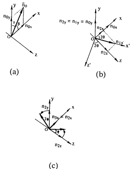
Fig. 2. Change in the unit normal vector  $\hat{n}$  of the reflected equiphase plane. (a) Unit normal vector  $\hat{n}_0$  at  $\theta = \phi = 0$ . (b) Rotation of vector  $\hat{n}_0$  by angle  $\theta$  of the object. (c) Rotation of vector  $\hat{n}_2$  by angle  $\phi$  of the object.
