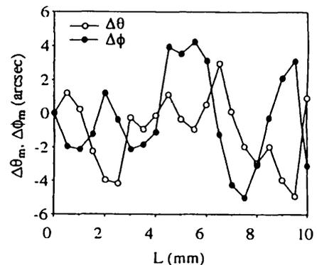
Fig. 10. Measurement results of 2D small rotation angles from displacements of a stage.
