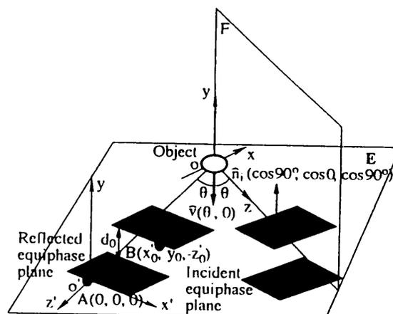
Fig. 3. Ideal configuration for measuring small rotation angle  $\Delta\phi$ .
