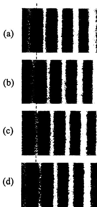
Fig. 6. Fringe images observed with the phase shift.
