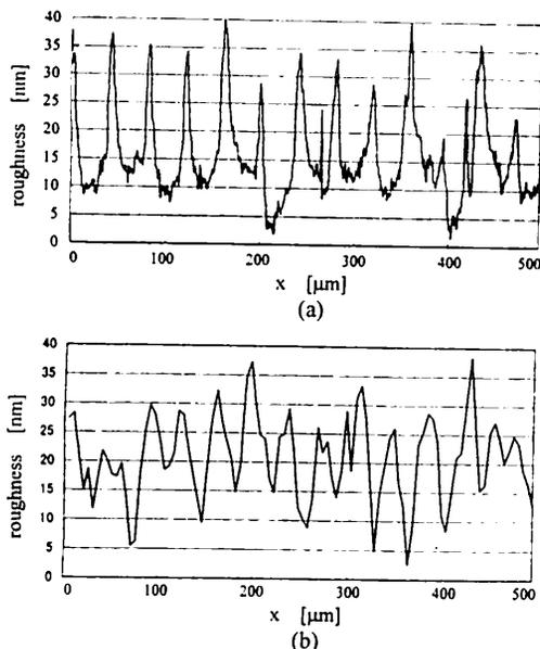
Fig. 7. Two-dimensional surface profiles of a diamond-turned aluminum disk measured with (a) a Talystep profilometer and (b) our system.
