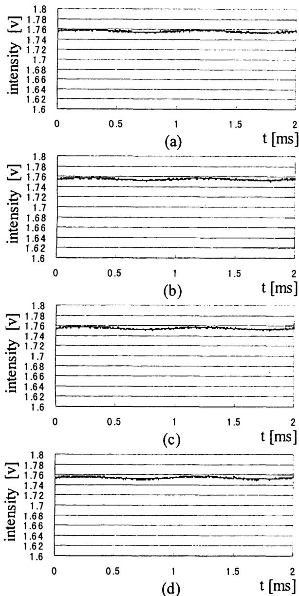
Fig. 5. Intensity change with photothermal modulation. The amount of phase shift is (a)  $\alpha_1 = 0$ , (b)  $\alpha_2 = \pi/2$ , (c)  $\alpha_3 = \pi$ , and (d)  $\alpha_4 = 3\pi/2$ .
