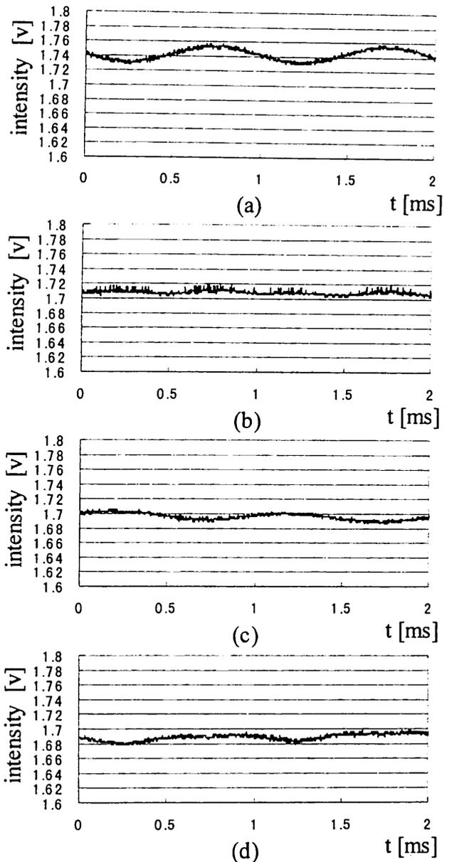
Fig. 4. Intensity changes caused by current modulation. The amount of phase shift is (a)  $\alpha_1 = 0$ , (b)  $\alpha_2 = \pi/2$ , (c)  $\alpha_3 = \pi$ , and (d)  $\alpha_4 = 3\pi/2$ .
