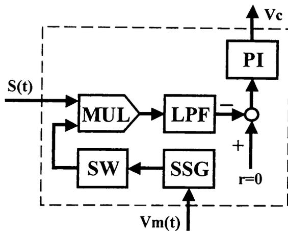
Fig. 2. Block diagram of the feedback controller. MUL, multiplier; PI, proportional-integral controller; other abbreviations are defined in text.
