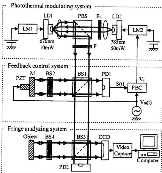
Fig. 1. Experimental setup: Abbreviations are defined in text.
